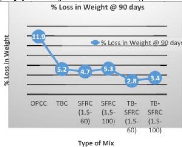
Loss of weight of specimens after immersion in 5% MgSo 4 solution for 90 days
